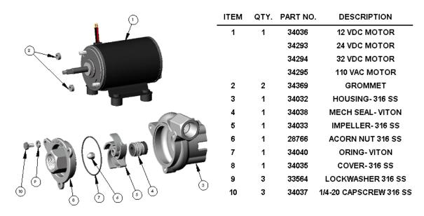
LS PUMP PSC MOTOR 3/4" NPT X 3/4" NPT
