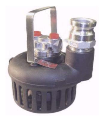
**HYDRASUB 20** is a compact, lightweight, hydraulically driven submersible pump with high flow capabilities. This self-priming pump is made with a high strength aluminum alloy that is anodized for corrosion resistance. This pump features a stainless steel impeller, ball bearing, and a gerotor type hydraulic motor.
