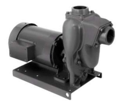
FLOMAX 8 self-priming centrifugal pumps are capable of creating vacuum sufficient to lift liquids from heights up to 25' above the source. Once primed the pumps built-in flapper valve will maintain a full column of liquid in the suction line.
