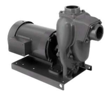
FLOMAX 5 self-priming centrifugal pumps are capable of creating vacuum sufficient to lift liquids from heights up to 25' above the source. Once primed the pumps built-in flapper valve will maintain a full column of liquid in the suction line.
