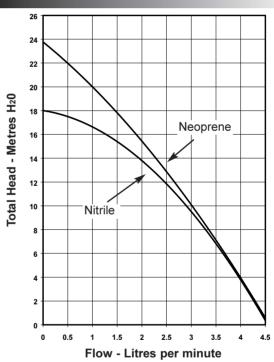
**Note**: Performance shown is for a new pump, pumping water at 20°C, performance may vary by up to 15%. Consult factory for performance of alternative impeller compounds.
