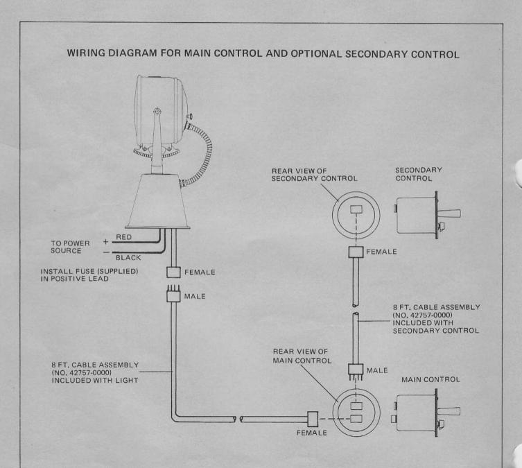
If additional cable is needed for main or secondary control connections, order 8 ft. cable assembly (no. 42757-0000) with mating plugs.
