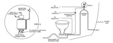
All runs of hose should be secured to a solid surface approximately every eighteen inches along the length of hose.
