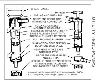
To reassemble pump, place disc valve in cylinder, snap intake cap back onto cylinder being sure undercut in cap is over cylinder roll. Insert plunger shaft assembly into cylinder and snap spout cap over cylinder roll.
