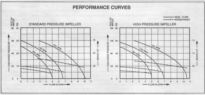
NOTE: Curves show approximate head flow for new pumps with neoprene impeller pumping water. Capacities should be reduced approximately 10% with nitrile and viton impellers.
