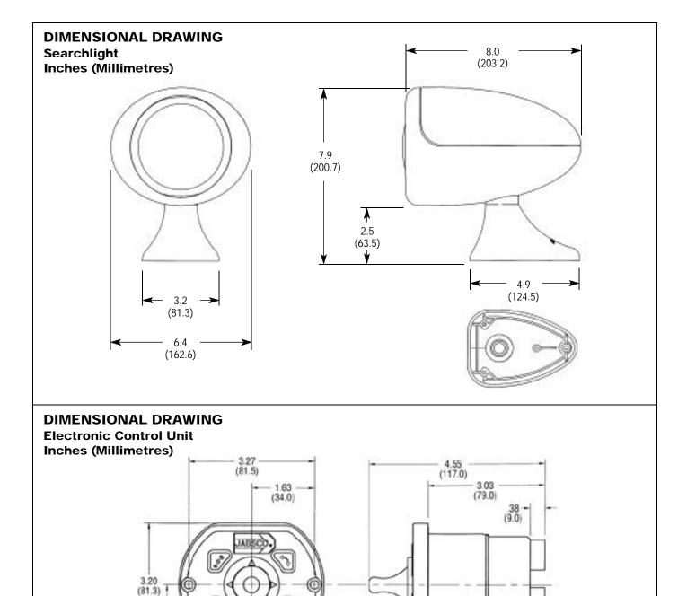
Mounting hole diameter 2.75" (70mm)
