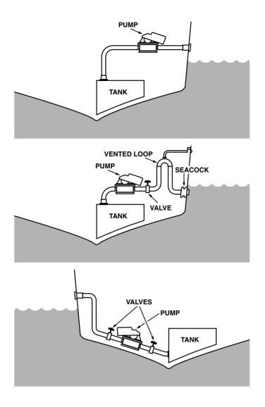
If the waste discharge plumbing can not be connected to a thru-hull positioned above the water line, the discharge plumbing must be fitted with a 1-1/2" vented loop positioned to remain about 8" above the water line at all angles of heel and trim.
