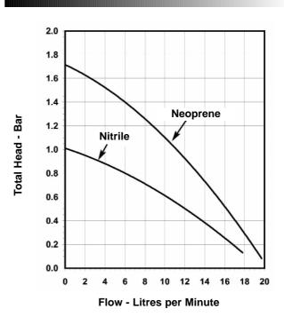
Note: Performance shown is for a new pump, pumping water at 20°C, performance may vary by up to 15%. Consult factory for performance of alternative impeller compounds.
