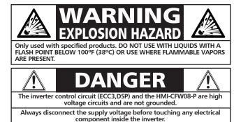
Many components are charged with high voltage and/or in movement (fans), even after the incoming AC power supply has been disconnected or switched OFF. Wait at least 10 minutes for the total discharge of the power capacitors.
