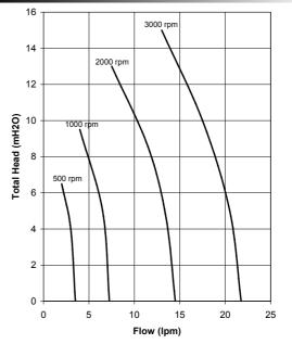
Note : Performance shown is for a new pump, pumping water at 20°C, performance may vary by up to 15%. Consult factory for performance of alternative impeller compounds.
