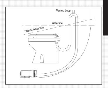
The vented loop fitting must be secured in a location that remains at least 6-8 inches (15-20 cm) above the waterline at all angles of heel and trim (see diagram).
