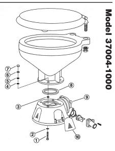
notch in the top of the base. Ensure the pump sealing O-Ring (gasket on very early models) is properly positioned in its groove (a little grease may be used to hold it in place) and carefully (so as not to dislodge the seal) slide the pump assembly into the base. Secure the pump to the base with the four machine screws and lock washers and torque each to 13-15 inch pounds.
