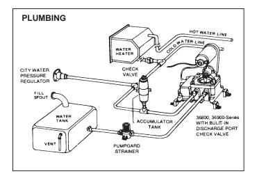
PRESSURE REGULATOR It is recommended that systems having a connection for a city water entry be equipped with a pressure regulating check valve set at approximately 35 psi. This valve automatically regulates the incoming water pressure to avoid damage to pump and plumbing from excessive pressures. Models 44410-Series (Permanent Flush Mount) and 44410-1010 (in-line Hose Type) pressure regulating valves are recommended for this purpose.
