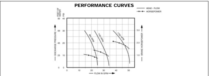
NOTE: Curves show approximate head flow for new pumps with neoprene pumping water.
