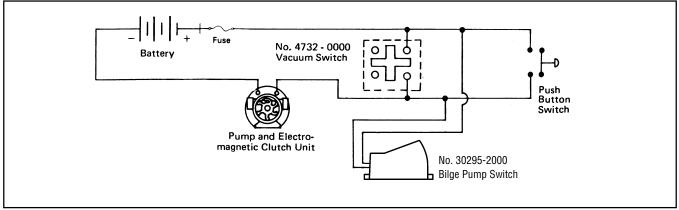
**REMOTE CONTROL** (When Engine Is Running): Install a pushbutton switch at one or more locations. Depress pushbutton for 2 seconds. If there is water in bilge, pump will operate until dry at which time vacuum switch will stop pump. If no water is in bilge, pump will stop when pushbutton is released.
