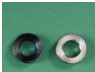
Valve Seats 17-4 PH Stainless Steel Tungsten Carbide Nitronic 50
