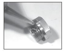
Remove the o-ring (31). Inspect all parts for wear and replace as necessary. Apply one drop of loctite 243 to the valve plugs (32) and tighten to 125 lb-ft (170 Nm)
