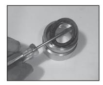
Remove the weep grooved seal (23) out of the seal adaptor (20). Check O-rings (21).
