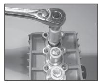
10) If the plunger pipe (16B), or oil seal (19) is worn, remove tension screw (16D) and remove along with plunger pipe (16B). Check and clean plunger surface (16A), check oil scraper (16H). Remove the seal case (20) and, if necessary, replace oil seals with seal lips facing crankcase (1).Cover thread of tension screw (16D) with a thin film of Loctite and tighten carefully to 221-265 in-lbs (25-30NM).
