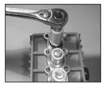
10) If the plunger pipe (16B), is damaged or worn, remove tension screw (16D) and plunger pipe (16B). Check and clean plunger surface (16A) and check flinger (16H). Cover thread of tension screw (16D) with a thin film of Loctite and tighten carefully to 22 ft.-lbs. (30NM).
