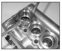
6) Remove seal adapters (20) and weep return rings (25) from the valve casing.
