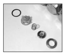
Remove each o-ring (#31). Inspect all parts for wear and replace as necessary. Reassemble valve assy's (32X) & place in valve casing (26).
