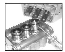
Remove weep return rings (#25) from the plungers (#16). Remove the seal case (#20) from either crankcases (#1) or manifold (#26) by using a screwdriver as shown above. NOTE: If there are deposits of any kind (i.e., lime deposits) in the valve casing, be certain the weep holes in the weep return ring (#25) and valve casing (#26) have not been plugged.
