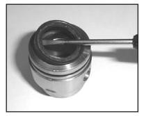
10. Remove the weep grooved seals (23A for all pumps except P318/P32 & #23 for P318/P324 only) from the seal case (#20).
