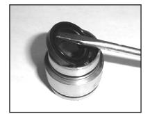
12. For all pumps (except P318/P324), use a flat screw driver to pry the oil seals (#19) loose from the seal case (#20).
