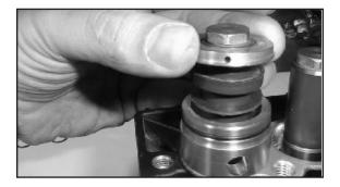
15. Place each seal case (#20) with o-rings (#21, 22) over the plungers (#16). Be certain the oil seal is centered with the seal case and tap firmly until the seal case is seated squarely on the crankcase (#1). 16. With the grooved side pointed toward the valve casing, place the weep grooved seals (23A for all pumps except P318/ P324 & #23 for P318/P324 only) over each plunger and into each seal case (#20).
