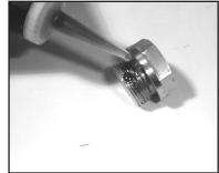
5. Apply one drop of Loctite 243 to valve plugs (32) and tighten to 59 ft.-lbs. For pumps manufactured prior to 5/97 tighten plugs to 37 ft-lbs.
