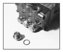
With a 24mm socket wrench, remove the (3) discharge valve plugs and (3) inlet valve plugs (#32). Inspect the o-ring (#33) for wear and replace if damaged.
