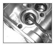
Remove the pressure rings (#24) and grooved seals (#23) from the valve casing (#26). Inspect parts for wear and replace if necessary. For P318 & P324 only, the spacers (#23A) can now be removed.
