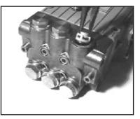
Using a needle nose pliers, remove the inlet and discharge valve assemblies (#32X).
