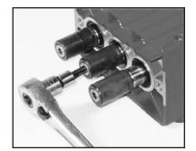
13A. **P318/P324 Only!** Clean the old sealant from the threads of the tension screw and the plunger base (16A). Place plunger pipes over plunger base and secure with tension screw to 220 in-lbs.
