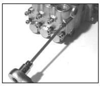
5. Next, use a 5mm allen wrench to remove the 8 socket head cap screws (34).
