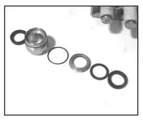
7. Remove the weep return ring (25), pressure ring (24), and v-sleeve (23) from the valve casing (26). Remove the v-sleeve (23A) from the seal case (20). Inspect all parts, including o-ring (21) for wear and replace as necessary
