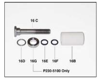
8. Check surfaces of plunger pipe (16B). A damaged surface will cause accelerated wear on the seals. Deposits of any kind must be carefully removed from the plunger surface. A damaged plunger must be replaced!
