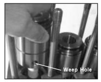
13) Replace complete seal sleeve (35)/seal case (37) assembly into crankcase (1). Make sure that the weep hole points downward. Note: To replace the oil seals (31), you will need to disassemble the gear end (see instructions below).
