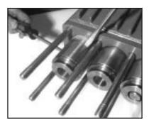
7) Remove the seal sleeve (35) from the manifold and /or crankcase.
