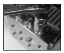
Loosen and remove tension plugs (48) with a 36mm socket wrench.
