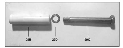
12) Check plunger surface (29B). If plunger pipe is worn out, loosen tension screws (29C) with a 15mm socket and pull off plunger pipe to the front. Clean front surface of plunger (29B) thoroughly. Apply a small drop of locktite to tension screw. Put a **new** crush washer (29D) onto tension screw. Put a thin coat of glue (Loctite) on the ring (or ceramic plunger side) and tighten screw to 265 in.-lbs.
