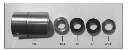
11) Remove the pressure ring (40A), v-sleeves (40), and support ring (40B), from the seal sleeve. For LP301A pumps, remove the pressure spring (41). Examine seals carefully and replace if worn. Clean surfaces of seal sleeves (35) which come in contact with the crankcase (1) and sealing surfaces of valve casing (43).
