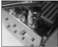
5) Tighten up tension plugs (48) to 107 ft.-lbs.
