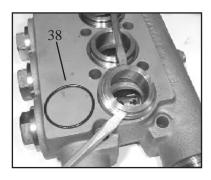
8. Remove seal case (37) from valve casing (43) and inspect o-ring (38).
