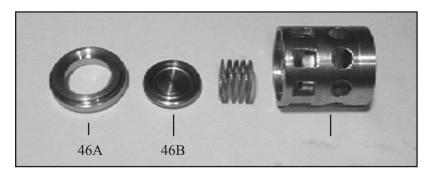
4. Loosen valve seats (46A) from spacer pipe (46D) by lightly hitting the valve plate (46B) with a plastic stick. Check sealing surface and replace worn parts. Reassemble with new o-rings (44A) and oil them before installing. Tighten up tension plugs (48) to 107 ft.-lbs.
