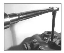
12. Place valve vasing (43) over studs and push firmly until seated against the crankcase (1). Tighten the hexagon nuts (49A) in a crosswise pattern (shown below) to 59 ft.-lbs.
