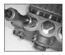
3. Remove the complete valve assembly (46) with valve pullers.
