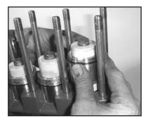
Press seal sleeve assembly into the manifold and seat firmly. Put the support ring (41) on plunger with v-side facing the manifold.
