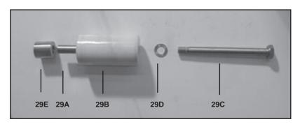
Inspect surface of plunger pipe (29B) carefully. Remove any chemical or mineral deposits taking care not to damage the surface of the plunger. If plunger pipe is worn, remove the plunger bolt (29C), plunger pipe (29B) and spacer (29E). Replace worn parts necessary. *Note: <u>Always</u> use a new copper gasket (29) when repairing the plunger assembly.*
