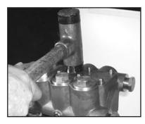
12. Place entire manifold/seal sleeve assembly over the studs and push firmly until seated against the crank-case.
