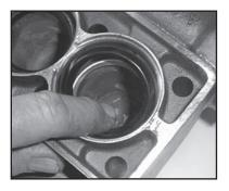
Place support ring (41) and v-sleeves (40) into valve casing. For LP250-3100, the support disc (37) is placed in the manifold before the support ring.
