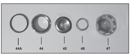
To disassemble the valve, screw the bolt into the retainer until the valve plate (45) presses the valve seat (44) out of the spring retainer. Examine all parts and replace if necessary. If the seat doesn't come out, use a valve puller to remove.
