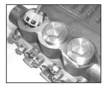
Next, place valve assemblies (46A) into manifold after first lubricating the O-ring (44A). Seat firmly into manifold.
