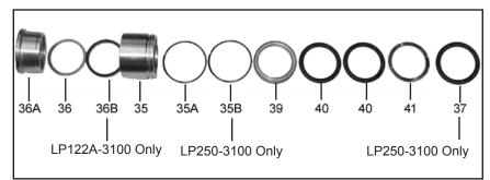
4. Remove the seal sleeve (35) from the manifold and/or crankcase. Remove the pressure rings (39 & 36A), drip shield for LP122A-3100 only (36B), v-sleeves (40 & 36), support ring (41) and o-rings (35A) from the manifold and seal sleeve, respectively. LP250-3100 pumps also have a support disc (37) and an O-ring (35B) for the seal sleeve. Examine seals carefully and replace if worn. Clean all parts.
