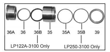
Lubricate seal (36). Place seal (36) and drip shield (36B for LP122A-3100 only), and pressure ring (36A) into the seal sleeve (35). Assemble the O-ring (35A) onto seal sleeve and lubricate. LP250-3100 has an additional O-ring (35B).
