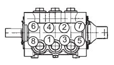
13. Tighten hex nuts (49A) in a crosswise pattern (shown above) to 60 ft.-lbs. (81 Nm).
