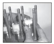
Oil seal replacement can be accomplished by pulling the retainer forward out of the crankcase. The O-ring around the outside of the retainer should be replaced and lubricated with a light film of oil.
