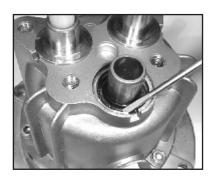
12. If the crankcase oil seals (15) are to be replaced, they can be removed by prying loose with a screwdriver. Take care not to make contact with the plunger (8) and pry out the oil seals from their housing. Seals should not be reinstalled until after step
