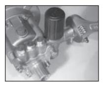
3. With a crescent wrench, remove the kickback valve spring retainer (47). Inspect the o-ring (46) for wear and replace as necessary. Remove the kickback valve spring (43), kickback valve cone (42), and the o-ring (41) from the manifold (35). Inspect the parts for wear and replace as necessary.
