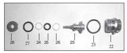
Remove the piston (24), o-ring (26), and backup rings (25). Remove the bypass valve seat (28). Inspect the parts for wear and replace as necessary. IMPORTANT! Make sure that the shoulder on bypass valve seat (28) is facing the discharge plug (22).
