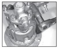
6. With a 14mm socket wrench, remove the guide plug (22) and o-ring (23).
