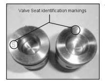
7) When reassembling: The inlet valve seat (51C) is 1mm smaller in diameter than the discharge valve seat (52C). Inlet valve seats are marked "S" and always have to be installed first. Discharge valve seats are marked "P" and are always to be installed on top of inlet valve. Plugs (58) are to be tensioned down evenly with screws (58C) and in crosswise pattern at 155 (ft.lbs.).
