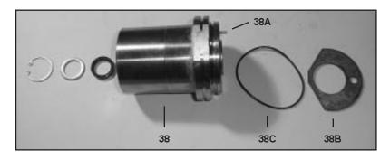
15) Remove leakage gasket (38B) from serrated pin (38A) on the seal sleave (38). Check o-ring (38C) for damage and replace if necessary. **IMPORTANT!** The 3.2 mm (diameter bore of the leakage gasket (38B) must be inserted directly on the serated pin (38A) of the seal sleeve (38). The leakage gasket must fit snugly to the seal so that the bevelled surface of the gasket faces outwords.
