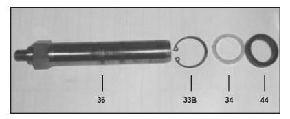
17) Examine plunger (36) for signs of wear or cavitation. If the surface of the plunger is worn, screw out the plunger with a 27mm tool. Clean centering and front surface of crosshead with plunger (25). Thread new plunger carefully through oiled seals in seal sleave. Coat thread of new plunger lightly with bonding agent (e.g., loctite).
