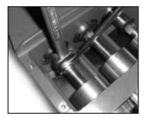
11) By gripping hex flats, separate plunger (36) from crosshead (25) by means of two open-end wrenches (size 22mm and 27mm).
