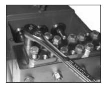
Lossen and remove screws (58C) with a 24mm socket wrench.
