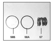
3) Remove the compression spring (57) O-Ring (58A) and support ring (58B).
