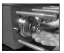
12) Remove tension spring (40) from seal retainer (38).
