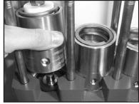
Place new plunger pipe (29B) carefully through the oiled seals and push seal sleeve (35) with plunger pipe into the crankcase guide. Note: Make sure weep hole is facing down.
