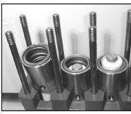
5. Pull seal sleeves (35) out of guides in crankcase (1).
