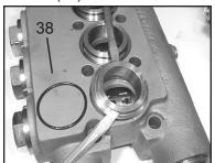
7. Remove seal case (37) from valve casing (43) and inspect o-ring (38).
