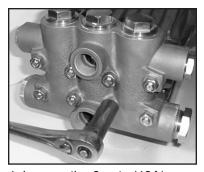
4. Loosen the 8 nuts (49A) with a 19mm wrench. Tap the back of the manifold (43) with a rubber mallet to dislodge and slide off the studs (49).
