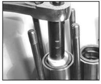
10. Tighten the tension screws (29C) to 310 in.-lbs. The plunger pipe (29B) should not be strained by over tightening of the tension screw (29C) or through damage to the front surface of the plunger; otherwise, it will probably break.
