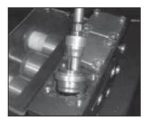
Remove spring (51C) and valve plate (51B). The seal ring (51E) is snapped onto the valve plate. Check sealing surfaces and O-rings (51F/57). Replace worn seals.
