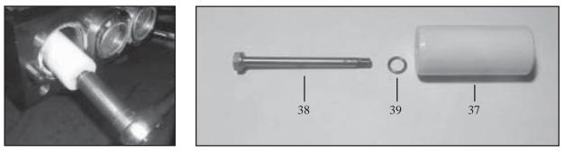
**IMPORTANT:** If plunger pipe (37) is worn, tap the tension screw (38) lightly with a plastic hammer beforehand to loosen the glue on the threads of the tension screw. Then screw out tension screw and remove the plunger pipe from centering sleeve (36). Using the tension screw put the new plunger pipe and a new copper ring (39) onto the centering sleeve. Cover the threads of the tension screw lightly with loc-tite and tighten to 30 ft-lbs.
