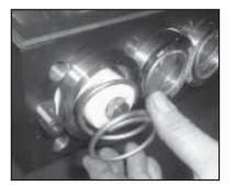
6) Take tension spring (42) out of seal sleeve (40).
