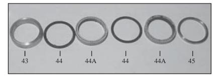
8) Remove seal unit (43, 44, 44A, 45) from seal sleeve. Examine packing rings (44A) and guide ring (43). Remove seal case (41) from valve casing and check O-rings (41A). Replace worn part, apply silicon grease on seals and O-rings before installing.
