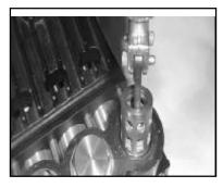
2. Remove discharge and suction valves (46), by pulling them upwards out of the valve casing with a valve puller.
