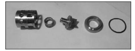
4. Unscrew the valve seat, remove the valve plate (46B) and spring (46C). The seal ring (46E) is snapped onto the valve plate. Check all sealing surfaces and replace worn parts. Tighten plugs (48) to 107 ft-lbs.
