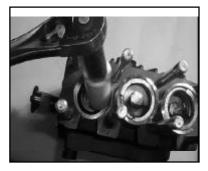
10. Remove tension screw (29C) and remove the plunger pipe from centering sleeve (29A)
