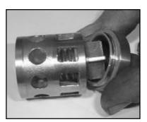
3. The spacer pipe (46D) is screwed together with valve seat (46A).
