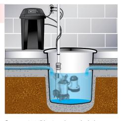
Operates in 14" basin or larger. Includes: Battery case control unit, 12V pump, Reed switch, AC Power supply, Wireless gateway, 1/2 HP primary pump - w/vertical switch, preplumbed w/wye connection & check valves
