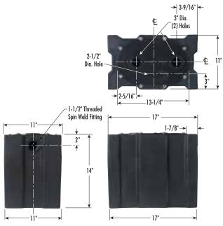
All dimensions in inches. Component dimensions may vary  $\pm$  1/8 inch. Dimensional data not for construction purpose unless certified. Dimensions and weights are approximate. On/Off level adjustable.
