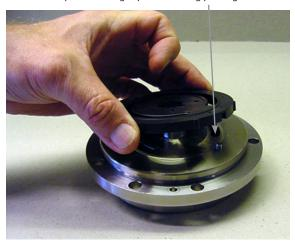
5. Mount housing using pin as guide.
