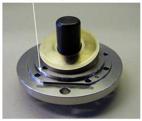
20. Mount washer and screw in front flange to fix swash plate.
