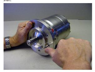
23. Mount front flange on te housing using pin as guide.
