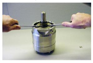
Remove guide pin from housing and the two guide pins from swash plate.
