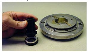
14. Mount ceramic ring by pressing tool as far down in front flange as possible.
