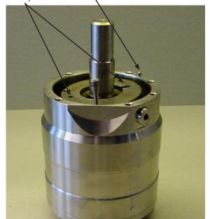
7. Remove swash plate using the 4 mm front screw.
