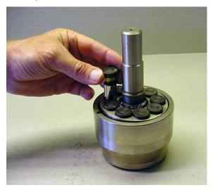
14. Remove retaining plate.
