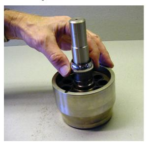
16. Remove thrust plate using two screwdrivers.
