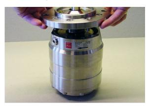
5. Remove shaft seal using two screwdrivers.
