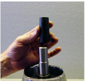
25. Tighten screws to a torque of 30 Nm and mount parallel key on shaft.
