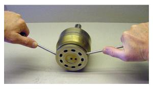
17. Remove shaft sealing from front flange.
