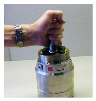
9. Unscrew the eight screws M8 in port flange (6 mm key).
