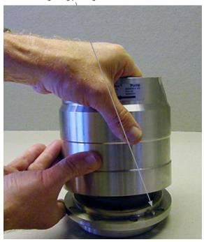
5. Place housing and port flange near table edge and mount screws from below.
