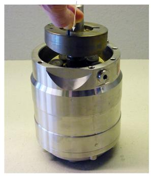
8. Remove cylinder barrel from housing.
