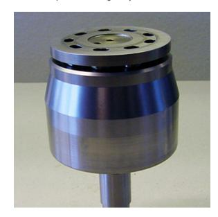
8. Press thrust plate into cylinder barrel using a table or the like as support.
