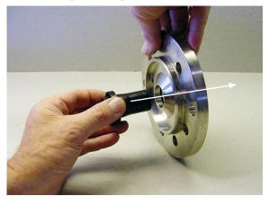
16. Mount shaft seal (carbon surface pointing downwards), spring, and washer (edge pointing downwards) by sliding them over the tool.
