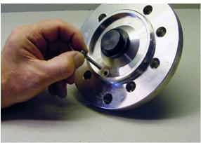
21. Tighten screw to a torque of 8 Nm and remove tool.
