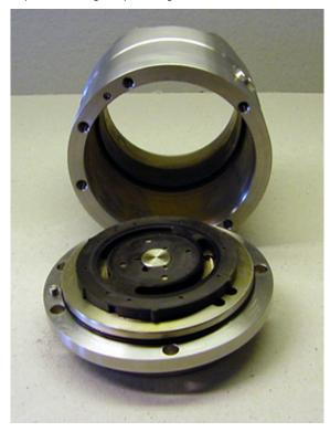
11. Remove valve plate from port flange.
