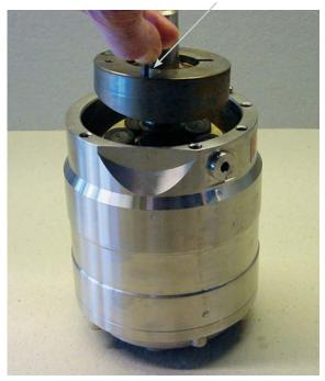
8. Remove the cylinder barrel from the housing.
