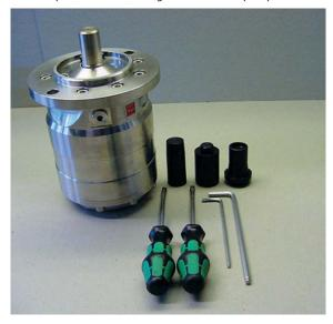
2. Remove the parallel key and unscrew the front screw.
