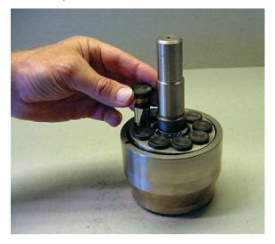
14. Remove the retaining plate.
