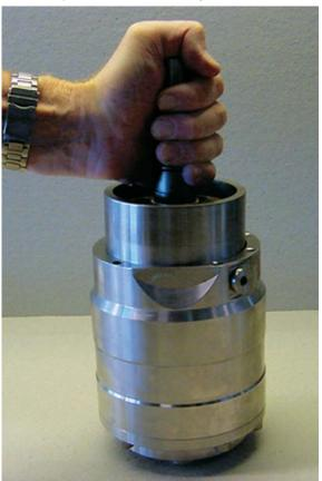
9. Slide the retaining ball (smallest diameter pointing upwards) down the shaft.
