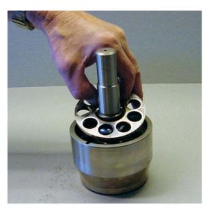
15. Remove the retaining ball.
