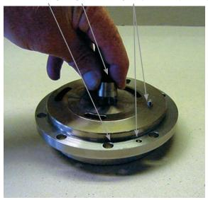
4. Mount the valve plate in its right position using the pin as guide.
