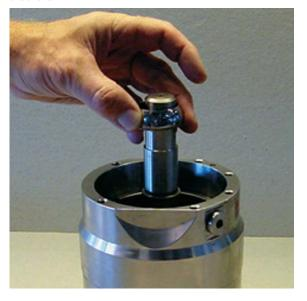
10. Mount the retaining plate (smallest centre diameter pointing upwards).
