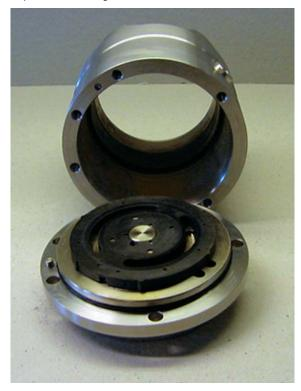
11. Remove the valve plate from the end cover.
