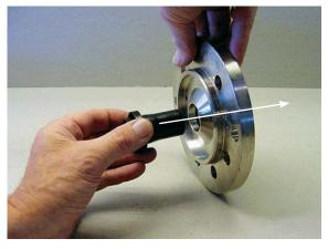
Mount the shaft seal (carbon surface pointing downwards), the spring, and the washer (edge pointing downwards) by sliding them over the tool.
