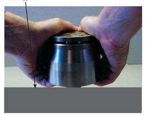
8. Mount the cylinder barrel in the housing.
