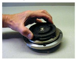
12. Remove the guide pins and the guide.
