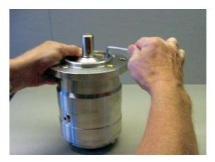
3. Unscrew the screws in the front flange.
