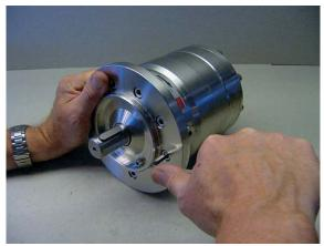
22. Mount the front flange on the housing using the pin as guide.
