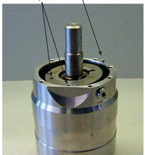
7. Remove the swash plate using the front screw.
