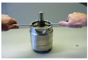
Remove the guide pin from the housing and the two guide pins from the swash plate.
