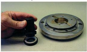
13. Mount the ceramic ring by pressing the tool as far down in the front flange as possible.
