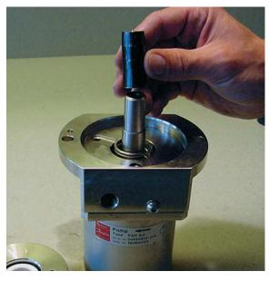
24. Mount the front cover and align it to the screw holes.
