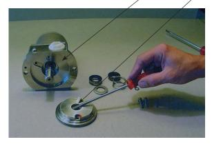
6. Unscrew the four screws for the housing.
