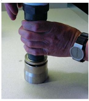
Check that the gap between the cylinder barrel and the thrust plate is 1.5-2.5 mm.
