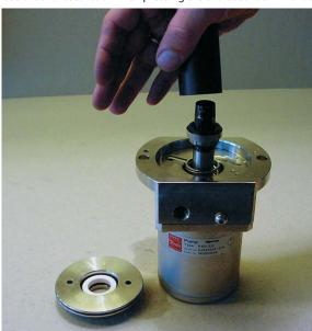
22. Press the shaft seal in position.
