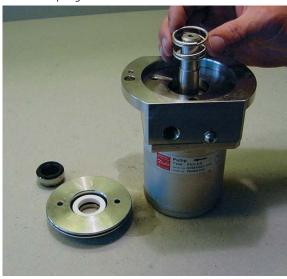
19. Fit the hollow bush onto the shaft.
