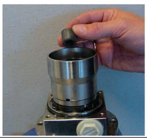
9.2.c. Mount the retainer guide on the spring guide.
