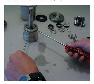
12. Remove the thrust plate.
