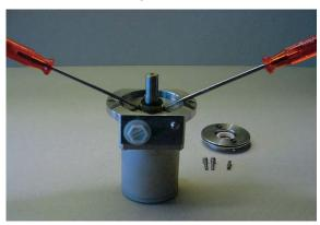
5. Remove the two small O-rings from the flange. Remove the seal from the front cover using a screwdriver.
