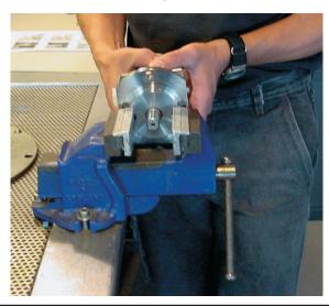
4. Remove the shaft seal using two screwdrivers.
