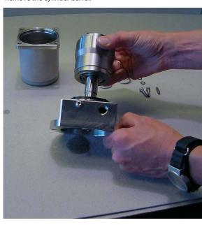
9. Remove the pistons and the retaining plate from the cylinder barrel.
