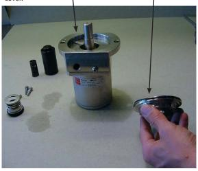
16. Wet the shaft seal with water and mount it in the front cover. Ensure that it is pressed to the bottom.
