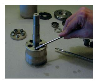
14. Remove the port plate from the flange.
