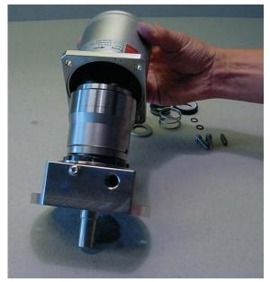
8. Remove the cylinder barrel.
