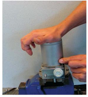
14. Tighten the screws to a torque of 13 Nm.
