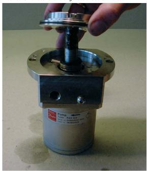
25. Tighten the screws to a torque of 7 Nm.
