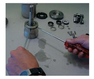
14. Remove the thrust plate.
