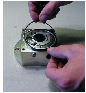
4. Mount the port plate in its right position using the pin as guide.
