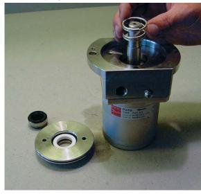
22. Fit the hollow bush onto the shaft.
