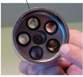
3. Ensure that the pistons can move freely in the bushings.
