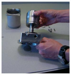
9. Remove the pistons and the retaining plate from the cylinder barrel.
