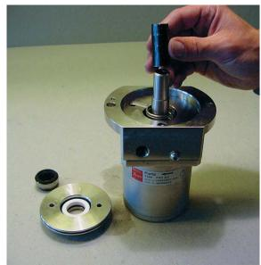
23. Wet the shaft seal and slide it over the bush.
