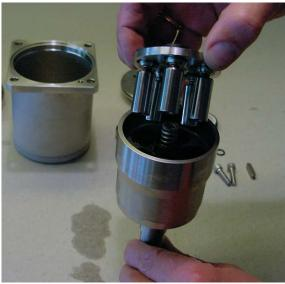
10. Remove the retaining guide.
