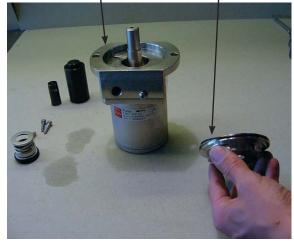
Wet the shaft seal with water and mount it in the front cover. Ensure that it is pressed to the bottom.
