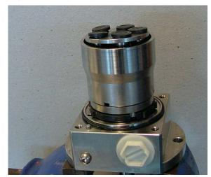
15. Mount the pump housing using the pin as guide.
