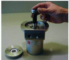
24. Use the shaft seal tool when pressing the shaft seal downwards.
