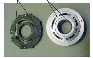
2. Hold a ruler against the surface of the plates and check the tightness against a light source.
