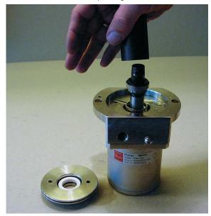
25. Press the shaft seal in position.
