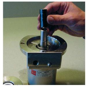
24. Mount the front cover and align it to the screw holes.
