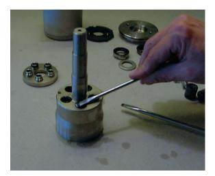
16. Remove the port plate from the flange.
