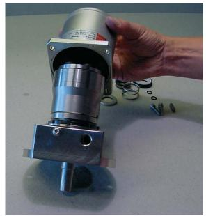
8. Remove the cylinder barrel.
