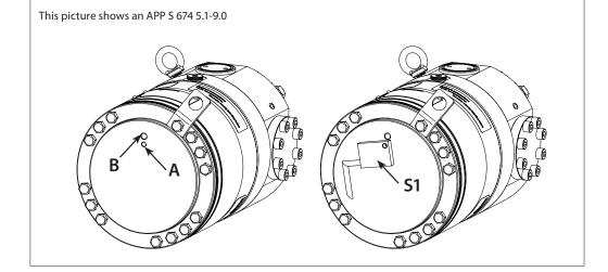
All APP S 674 pumps are designed with M6 and M8 threads for mounting the temperature sensor. The threads are placed differently depending on pump size.
