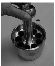
8. Carefully remove the valve plate assembly using a screwdriver.
