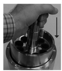
15. Fit the retaining ball onto the shoulder of the shaft.
