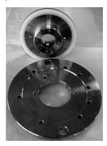
26. The mounting flange is now ready to be mounted on the housing.
