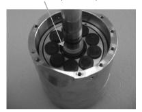
19. Mount the new shaft seal following the instructions in "Shaft Seal - APP 5.1 - 10.2" (521B0738).
