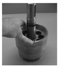
Position the new port plate over the guide pin.
