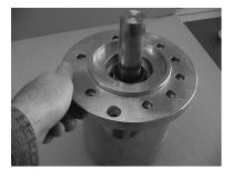
29. Screw the 8 screws into the flange and the housing.
