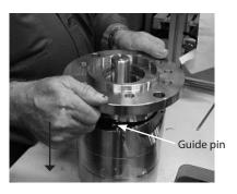
28. Position and carefully press, by hand, the combined flange and swash plate into the housing.
