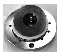
22. Remove the swash plate and the spacer.
