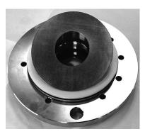
27. Position the guide pin in the housing.
