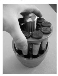
18. Position the new white spacer on top of the retaining ball.
