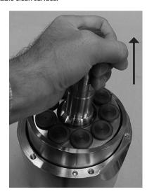
7. Remove the pistons, retaining plate, distance ring and retaining ball from the cylinder barrel.
