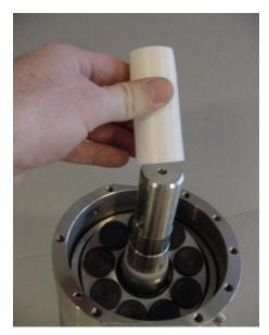
9. Thoroughly wet the torpedo, shaft and replacement shaft seal with plenty of soap. **Do not use silicone grease.**
