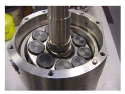
7. Scrap the old spacer (if black) and place the new white spacer on top of the retaining ball.
