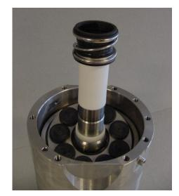
11. Use the plastic assembly tool provided, **large diameter pointing downwards**, to press the seal home against the shoulder of the spacer.
