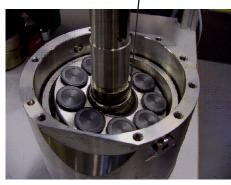
8. Fit the hollow bush (torpedo) onto the shaft.
