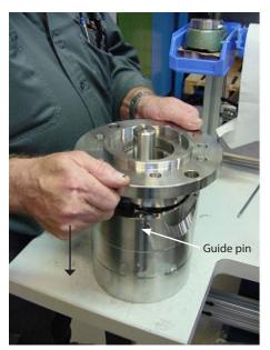
14. Screw the 8 screws into the flange and the casing. To prevent cold welding, lubricate the threads on the 8 screws with grease, screw them into the pump and tighten by hand. Use Molykote® D paste from Dow Corning or Klüber UH1 84-201 from Klüber lubrication.
