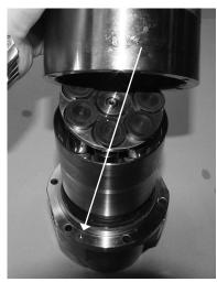
22. Hold pump together and carefully turn it over to rest on housing. To prevent seizing-up, lubricate the threads on the 2 screws and screw them into port flange and housing. Use Molykote® D paste from Dow Corning or Klüber UH1 84-201 from Klüber lubrication. Tighten the 2 flange screws to a torque of 12 +1 Nm.
