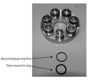
11. Wet O-rings and back-up rings with clean (filtered) soap-water.
