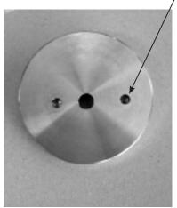
31. Screw centre bolt into centre of swash plate and tighten to  $6 \pm 1$  Nm.
