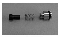
15. Press new spring onto shoulders of poppet guide and poppet so it is stuck on both collars. Then mount new O-ring on poppet guide.
