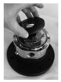
9. Gently lever valve plate assembly free with the aid of a screwdriver.
