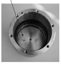
30. Carefully align swash plate over guide pin. Only one of the wholes fit /
