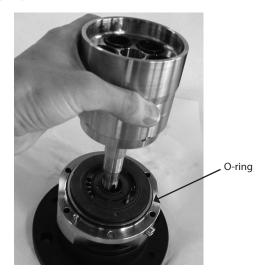
20. Position new spring, new spring guide, new retainer ball, new retainer plate and new pistons.
