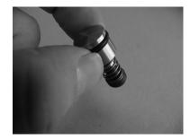
17. Mount flushing valve by pressing it into the hole.
