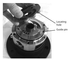
IMPORTANT: Make sure that guide pin is located in the locating hole in port plate.
