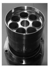
7. Remove cylinder barrel.
