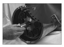
Place the retainer ring in an odd angle corresponding to the orientation of the swash plate.
