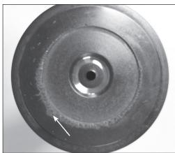
**Picture 3:**Cavitation of the piston shoes.
