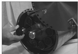
3. Remove the stop for retainer ball.
