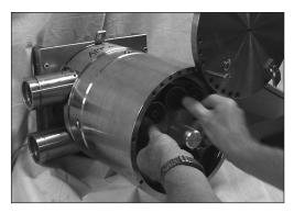
2. Lubricate pistons with clean filtered water Insert the pistons arbitrarily.
