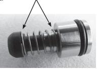
16. Turn flushing valve upside down. If not properly assembled, spring will fall off.
