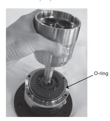
20. Position the new spring, new spring guide, new retainer guide, new retainer plate and new pistions.
