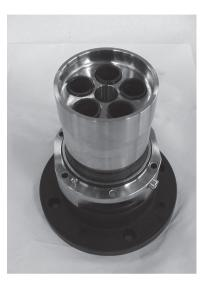
7. Remove the cylinder barrel.
