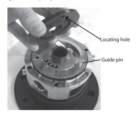
19. Replace the O-ring on the port flange and position the new cylinder barrel on the port plate.
