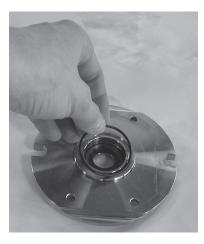
25. Lubricate the threads on the 4 screws with grease and screw them into the pump and tighten by hand. Use Molykote D paste from Dow Corning or Klüber UH1 84-201 from Klüber lubrication
