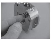
Position the port plate over the guide pin.
