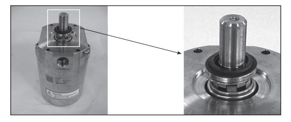
24. Replace the O-ring on the SAE flange
