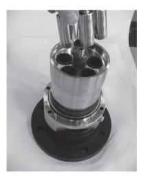
21. Position the housing on the port flange and over the guide pin.
