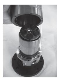
22. Hold the pump together and carefully turn it over to rest on the housing. To prevent seizing-up, lubricate the threads on the 2 screws and screw them into the port flange and the housing. Use Molykote D paste from Dow Corning or Klüber UH1 84-201 from Klüber lubrication. Tighten the 2 flange screws to a torque of 12+1Nm.
