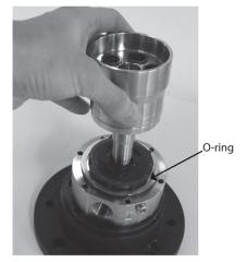
15. Position the new spring, new spring guide, new retaining ball, new retainer guide and new pistions.
