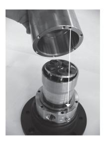
17. Hold the pump together and carefully turn it over to rest on the housing. To prevent seizing-up, lubricate the threads on the 2 screws and screw them into the port flange and the housing. Use Molykote D paste from Dow Corning or Klüber UH1 84-201 from Klüber lubrication. Tighten the 2 flange screws to a torque of 12+1Nm.
