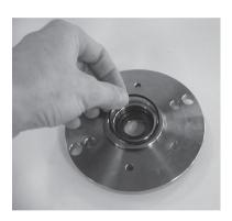
Lubricate the threads on the 4 screws with grease and screw them into the pump and tighten by hand. Use Molykote D paste from Dow Corning or Klüber UH1 84-201 from Klüber lubrication.
