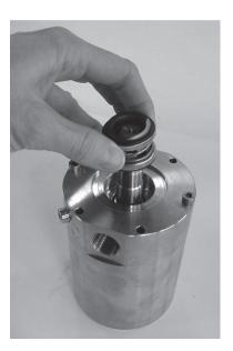
19. Replace the O-ring on the SAE flange.
