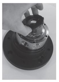
Gently lever the valve plate assembly free with the aid of a screw-driver.
