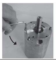
6. Remove the pistons, retaining plate, retaining ball, spring guide and spring from the cylinder barrel.
