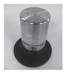
2. Wet the shaft and shaft seal with clean (filtered) soap-water. Gently lever the shaft seal assembly free using 2 screwdrivers.
