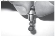
5. Mount flushing valve by pressing it into the hole.
