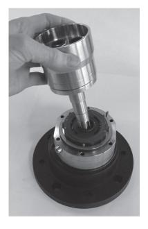
Remove the port plate and peek pin.
