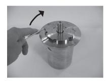
21. Tighten the screws to a torque of  $12 \pm 3$  Nm.
