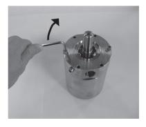
18. Mount the new shaft seal following the instructions in "Shaft Seal - APP0.6-3.5" (180R9089)
