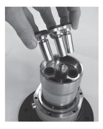
16. Position the housing on the port flange and over the guide pin.
