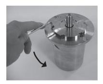
Carefully turn the whole pump over so that the shaft is facing down. Support the pump in a suitable hollow base so that the pump is not supported by the shaft.
