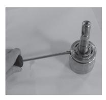
Replace the O-rings and the back-up rings on the valve plate.
