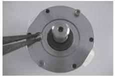
2. Assemble the new flushing valve, or replaced parts that are worn (shoulders)
