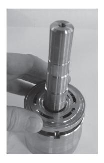
Position the port plate over the guide pin.
