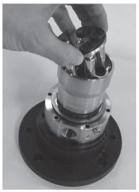
7. Remove the cylinder barrel.
