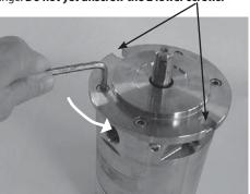
Wet the shaft and shaft seal with clean (filtered) soap-water.
