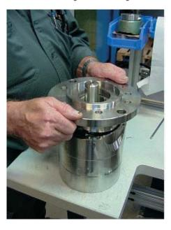
Screw the 4 screws into the flange and the housing. To prevent cold welding, lubricate the threads on the 4 screws with grease, screw them into the pump and tighten by hand. Use Molykote® D paste from Dow Corning or Klüber UH1 84-201 from Klüber lubrication.
