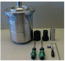
Unscrew the 4 mounting screws and remove the seal SAE flange. Do not yet unscrew the 2 lower screws.
