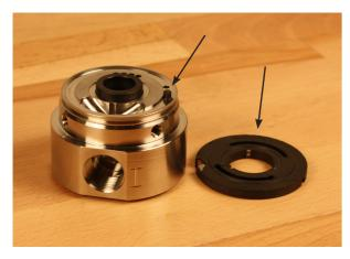
Warning This operation might break the shaft seal/bearing; this should thus only be done if it is broken and/or you have a new shaft seal set.
