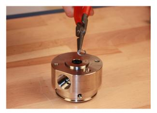
2. Use a small tool to push out the flush valve. (not sharp or pointed)
