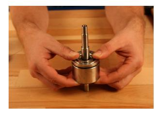
Lubricate the shaft with filtered soap water. Mount the cylinder barrel in the port flange. Use the torpedo in order not to damage the shaft seal by the sharp edge on the shaft.
