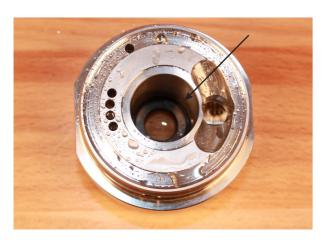
2. Mount the other part of the shaft seal. Make sure that the carbon ring is pointing towards the ceramic ring.
