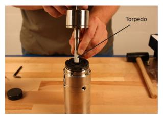
Lubricate the O-ring on the port flange with clean filtered soap water. Place the house on top of the port flange. Make sure to orient the port flange towards the holes in the house. Be careful not to squeeze the O-ring. Press down until it slides into place. Do not press on the shaft, as the cylinder barrel will be pressed out.
