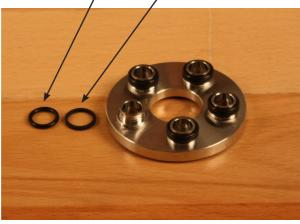
Wet the liners and O-rings/back-up rings with clean filtered soap water. Place the valve plate on top of the cylinder barrel and press gently downwards.
