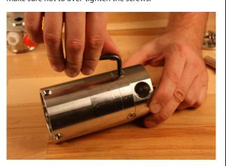
Mount the spring, retainer guide, retainer plate and pistons. Please confer with the exploded view at the end of this instruction for correct orientation. Warning: Ensure that the slant surface of the retainer plate is
