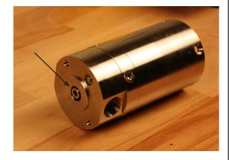
4. Gently lever the valve plate assembly free with the aid of a screw-driver
