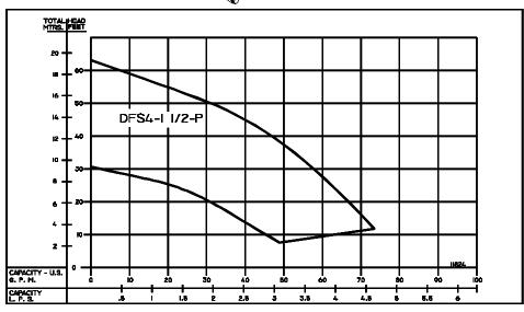
2900RPM - 50Hz. CAPACITIES TO 60GPM (3.8LPS) HEADS TO 43 FEET (13M)
